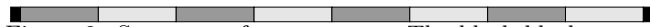
Figure 2: Structure of rec_fix.gz . The black blocks represent the header and the footer of the .gz file. The gray blocks correspond to stored (uncompressed) blocks and the light gray are compressed with the static Huffman table ( static blocks).
