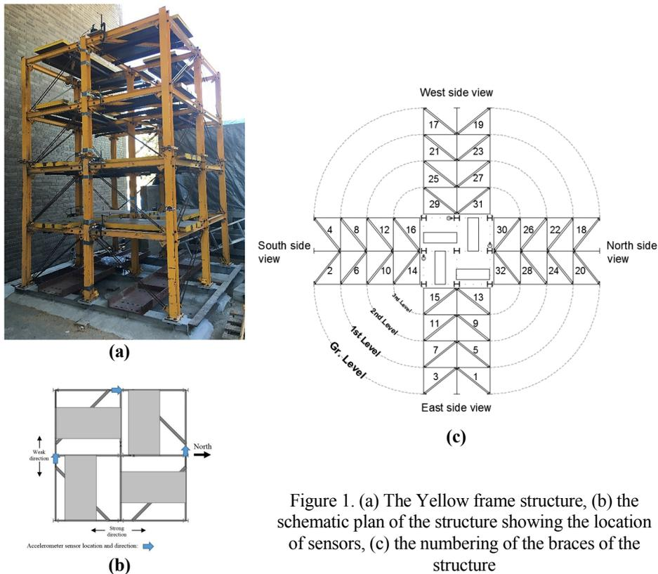
Figure 1. (a) The Yellow frame structure, (b) the schematic plan of the structure showing the location of sensors, (c) the numbering of the braces of the structure
