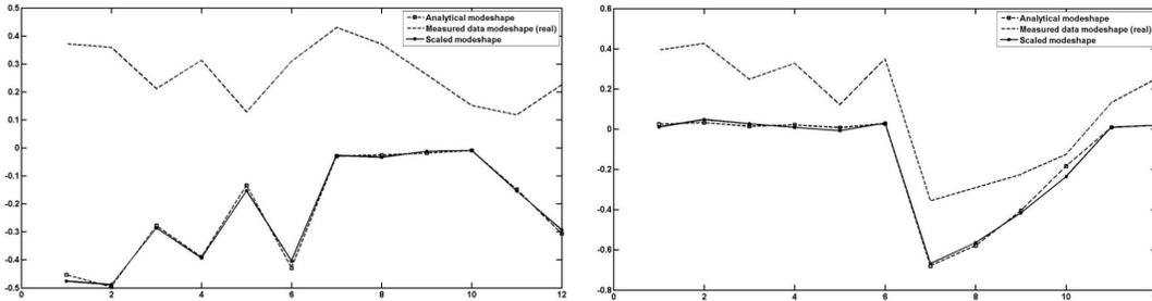
Figure 2. Mode shapes decoupling and scaling; (left: 1<sup>st</sup>, right: 2<sup>nd</sup> mode shape)
