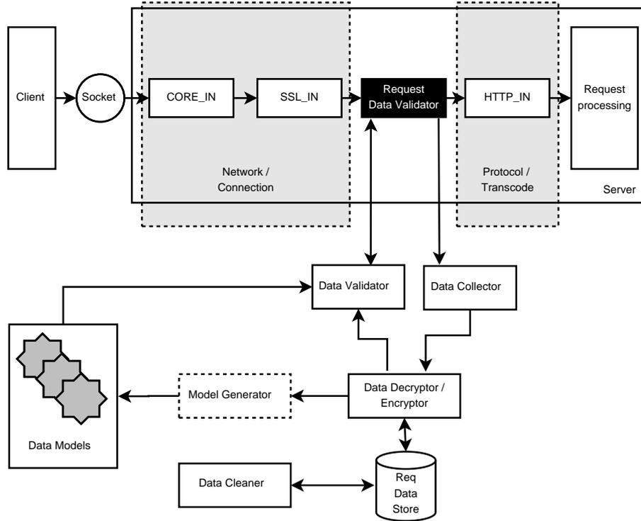
**Fig. 1.** The Learning Web Application Firewall components
