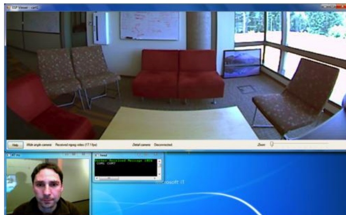
Fig. 3. View of the satellite’s interface. At the top is the view coming from the fixed wide-angle camera. The lower left window provides feedback of the image the satellite is projecting on his or her proxy. It also provides feedback that the head-tracker has a good representational model of the satellite’s head.
