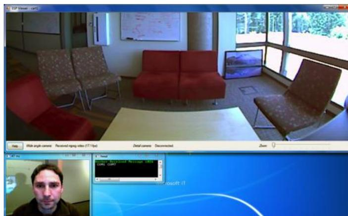
**Fig. 3.** View of the satellite’s interface. At the top is the view coming from the fixed wide-angle camera. The lower left window provides feedback of the image the satellite is projecting on his or her proxy. It also provides feedback that the head-tracker has a good representational model of the satellite’s head.
