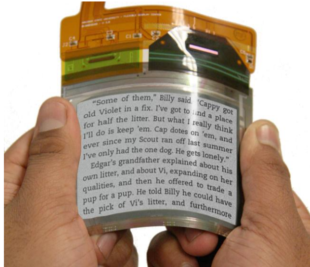
Fig. 1. E-ink Flexible Display
