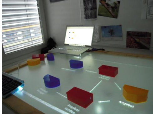
Fig. 1: System Overview, showing a simple procedural concept map on both, the table surface and the secondary display (computer screen)
