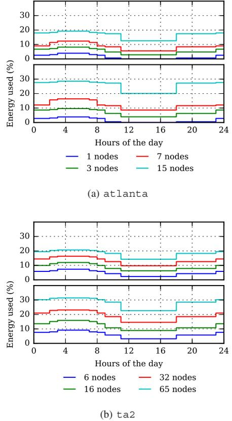
Fig. 3: Daily energy savings over the day for the (a) *atlanta*, and (b) *ta2* networks. with 10, 25, 50 and 100% SDN nodes deployment. Top plots: power model of the HP switch. Bottom plots: power model of an ideal energy efficient SDN switch.
