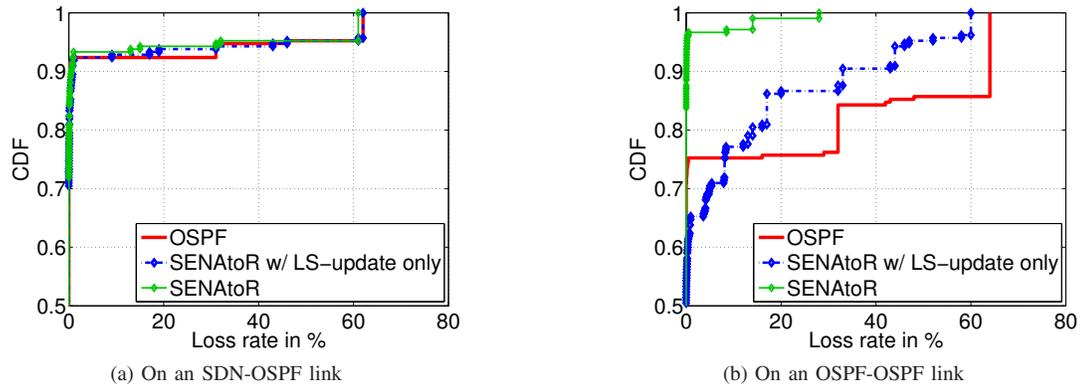
Fig. 6: Link failure experiment with the atlanta topology
