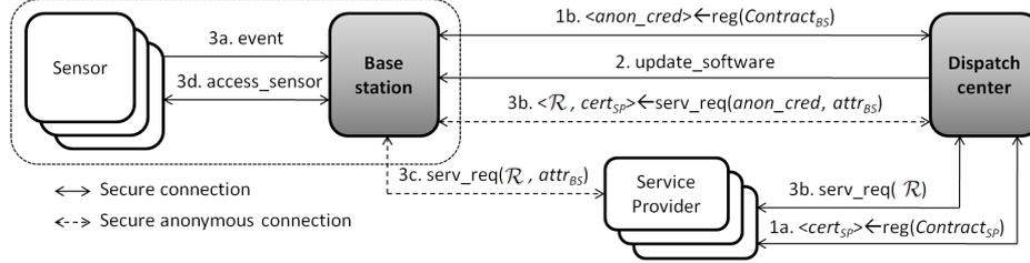
Fig. 1. Registration action and service consumption action
