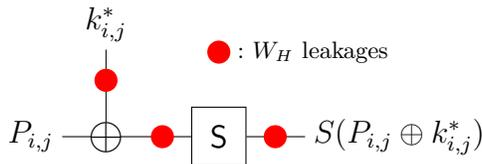
**Fig. 2.** Three interesting leakage points in the first AES round.
