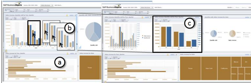
Fig 4. (a) Users select subset of their data, that get highlighted in all charts. (b) They drag their selections outside the chart to create a cut-out clone visualization (c), of the same type (here bar chart) with the selected data only. A blue highlighted bar (b) indicates the new chart will be placed on the right of the original, with existing charts shift to accommodate it (c).
