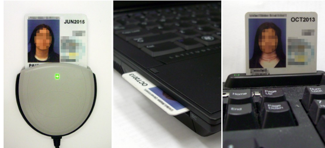
Fig. 1. From left to right: USB reader, laptop reader, integrated keyboard reader
