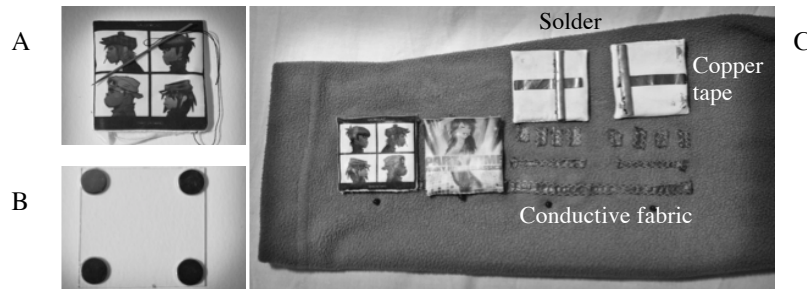
Fig. 2. Patch sensor A) front of final tag B) inner structure of tag showing rare-earth magnets at each corner C) jacket sleeve with conductive fabric; two tags are attached and two tags show circuitry on the back of the tags.
