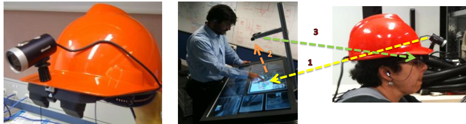
Fig. 1 Left: helmet with camera and near-eye display. Right: system work flow.
