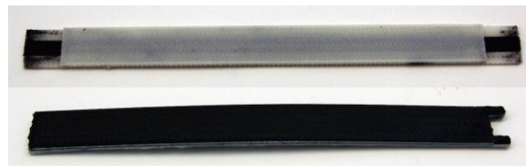
Fig. 9. Flex Sensors. Top: Single line method. Bottom: Elongated pressure sensor method.
