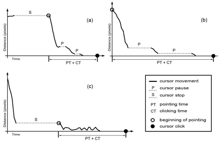
**Fig. 5.** Beginning of pointing trajectories estimations for 3 physically impaired participants using different computer pointing devices: (a) joystick, (b) numeric keypad with a head pointer and (c) oversized trackball.
