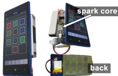
Fig 3. Phone-based CipherCard.
