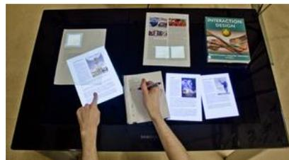
**Fig. 1.** ProjecTop system visualizing the occluded digital objects
