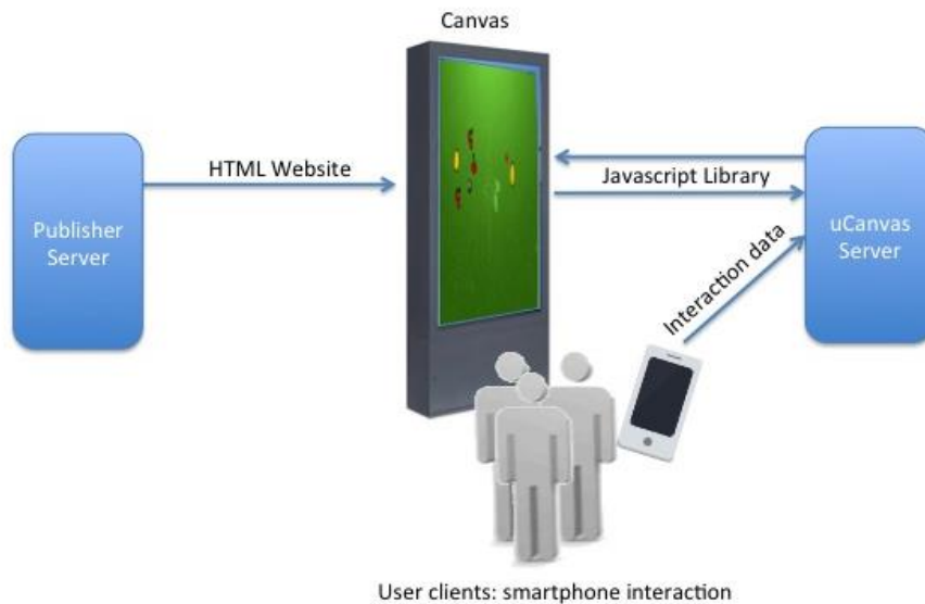
Fig. 2. A Javascript library connects publishers' content with the uCanvas server for interaction.
