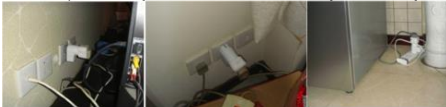
Fig. 1. Circle+ is connected to a television; circles is connected to a desktop and to a refrigerator (left to right)
