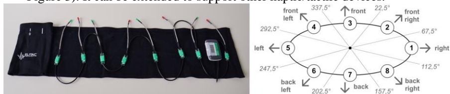
Figure 3. The tactile belt with 8 vibrators (the interval angel of each vibrator is 45°)
