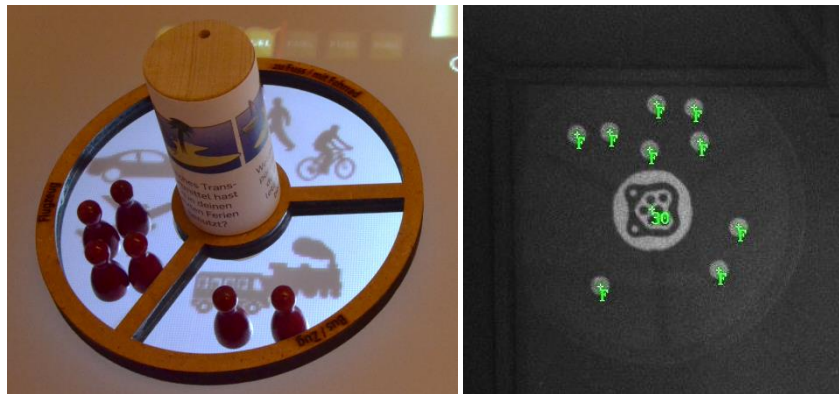
Fig. 2. The final design of the Tangible Voting widget (left); detection via reactIVision (right).
