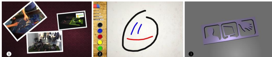
Figure 1. Three demo apps realised with TUIOFX in a few lines of code (LOC): (1) a multi-user video viewer (~100 LOC), (2) a drawing app (~450 LOC), and (3) a 3D model viewer (~400 LOC).
