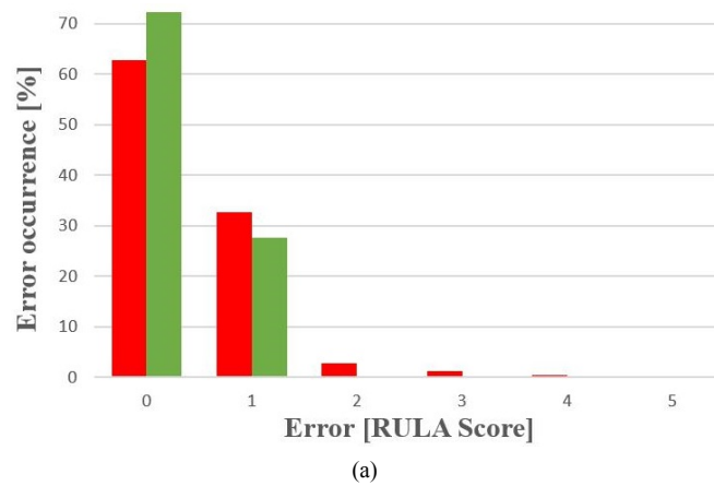
Figure 5 Histogram showing the percentage of frames for which the RULA score error is 0, 1...5 when using raw (red) and corrected (green) Kinect data (see online version for colours)
