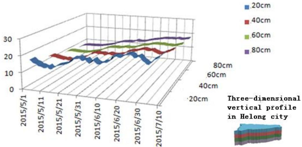
Figure 6 Vertical distribution of soil temperature Content
