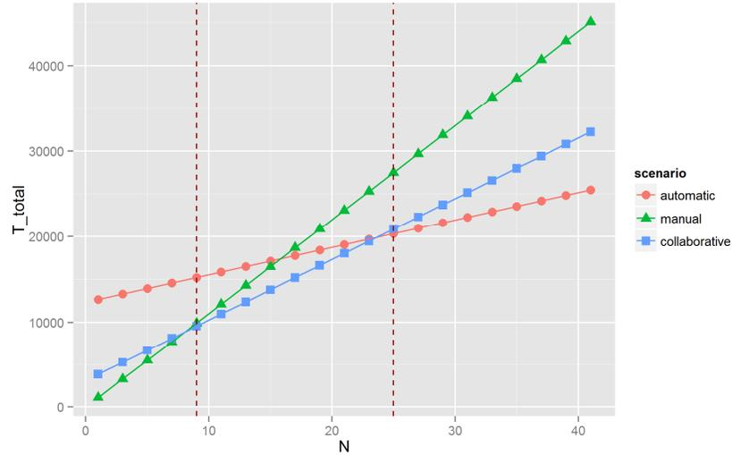
**Fig. 3.** Comparison of the total times in the three scenarios showing the range of the batch size in which the collaborative scenario is the most efficient.  $K = 10$ .
