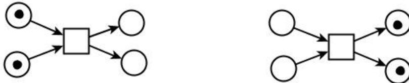
Fig. 3. Firing of a transition (before and after).
