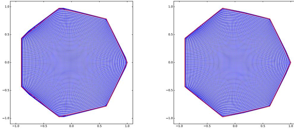
Figure 4: Mapping a square to heptagon. Left: stencil width = 4. Right: stencil width = 8.
