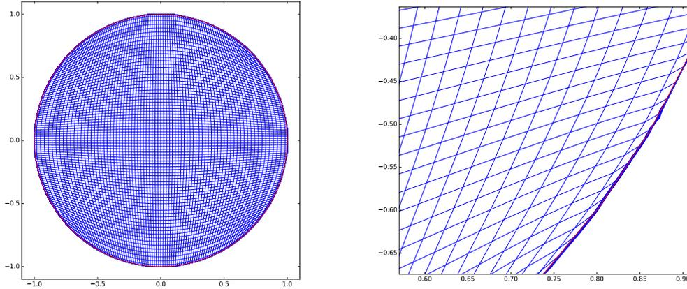
Figure 2: Left: Map deformation of the cartesian grid for square to ball test case. Right: Zoom of the Map deformation of the cartesian grid (test case to see  $D \setminus X$  mapped to  $\partial Y$ . Only the position of the grid points is really significant...)
