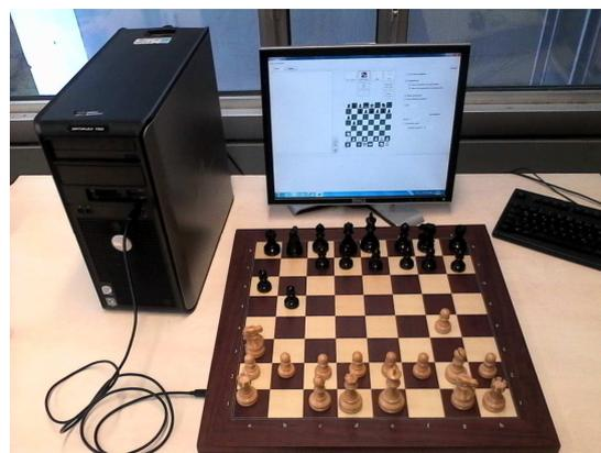
**Figure 1.** DGT electronic chessboard connected via USB to a computer.
