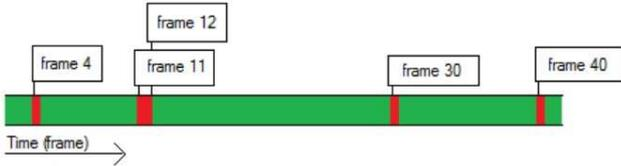
**Figure 4.** The traffic light shows the single frames of the scene video along the time axis. Each frame is represented as a small and vertical line. If the automatic annotation for a frame was successful, the line is drawn in green, otherwise in red (i.e. when the chessboard could not be automatically detected or if the fixation is not on the board). In this example, only frames 4, 11, 12, 30 and 40 could not be processed automatically and still have to be manually post-annotated.
