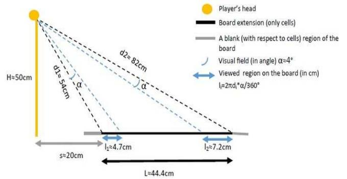
**Figure 7. Sketch for the calculation of the field of view in cm on the board ( $l_1$  and  $l_2$ ) from the field of view in angle ( $\alpha$ ), the distance of the player's head to the board plane ( $H$ ) and the distance between the player and the fixated cell on the board (variable from 10cm to 54.4cm).**
