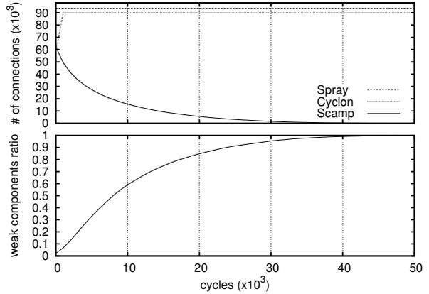
Figure 12: Number of arcs and partitioning in networks subject to failures in the connection establishments.
