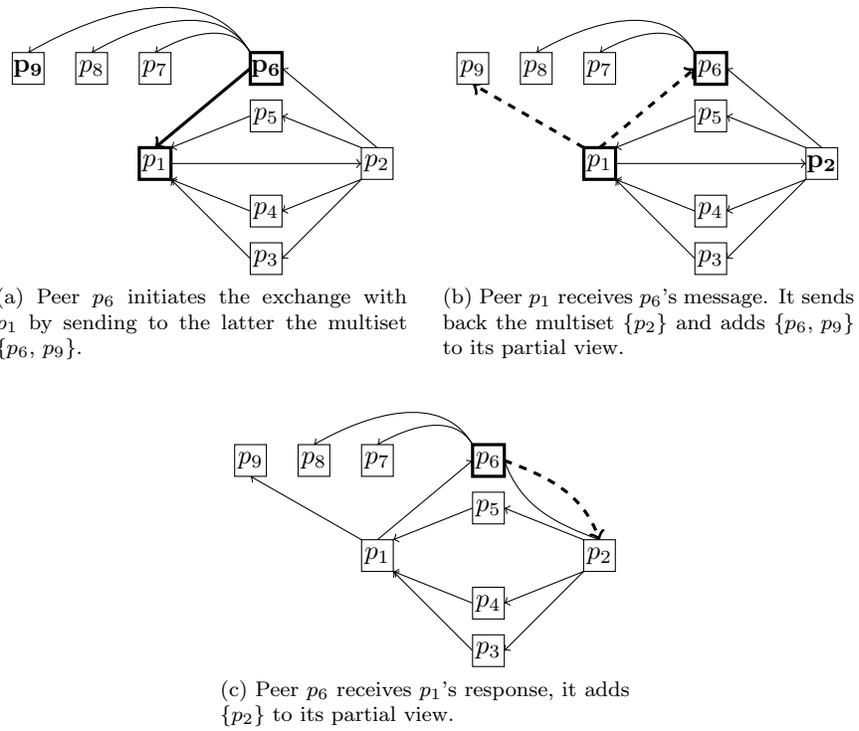
Figure 3: Example of the shuffling protocol of SPRAY.
