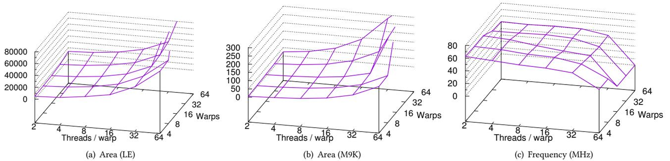
Figure 3: Simty scaling on Altera Cyclone IV as a function of threads per warp  $m$  and warp count  $n$ . Frequency is the worst-case estimate at 85°C in MHz. Area is given in Logic Elements (LEs) and in  $128 \times 32$ -bit RAM block (M9K) count. Place-and-route fails on configurations with  $\{16, 32, 64\}$  warps  $\times$  64 threads as a result of routing congestion.
