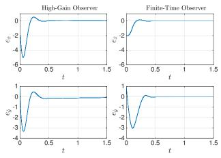
Fig. 1. Simulation plots of  $e_{\dot{x}}$  and  $e_{\dot{\theta}}$  for the HG and FT observers applied to the nonlinear plant with IC  $x(0)=(0,-2,\frac{\pi}{4},1)$  and  $K_n=10$ .
