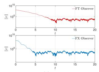
Fig. 4. Simulation plot of  $\|e\|$  for the FT and FX observers with measurement band limited noise to the linearized plant with IC  $x(0)=10^3(0,1,\frac{\pi}{4},0)$  and  $K_p=5$ .
