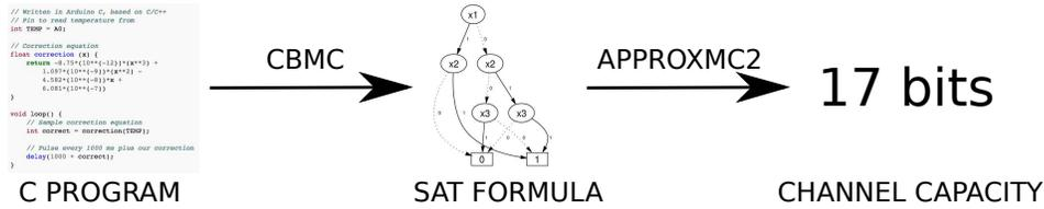
**Fig. 1.** A high-level view of ApproxFlow’s toolchain.
