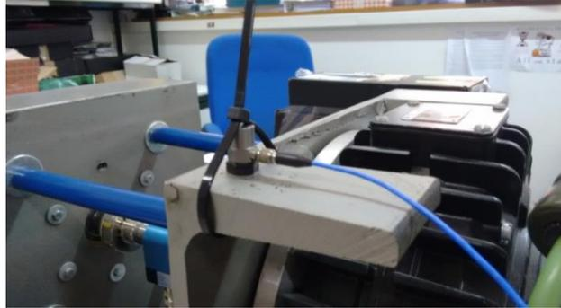
Fig. 4. Transversal vibrations measuring using an accelerometer.
