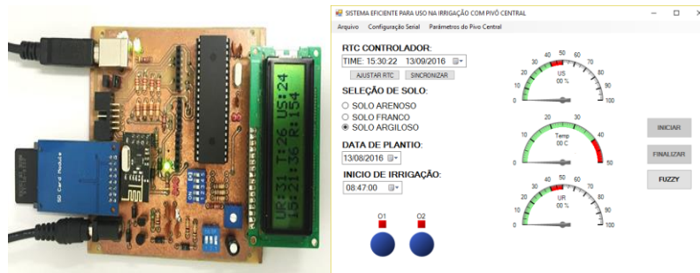
Fig. 5. Irrigation System Controller ( left ) and supervisory control software ( right ). The operator can adjust parameters from the irrigation mechanism on software.
