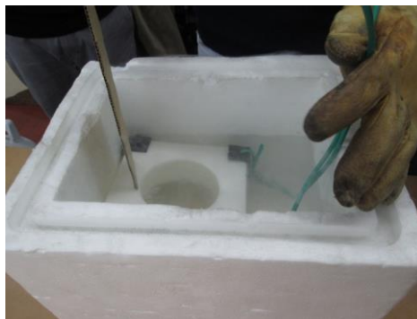
Fig. 4. Totally submerged stator in LN 2 .
