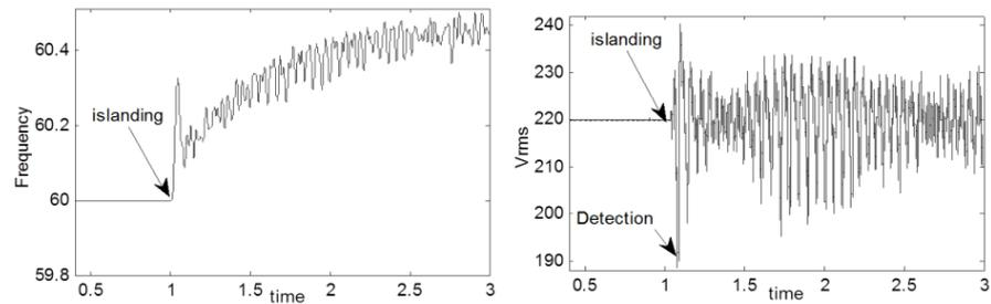
Fig. 5. Voltage and frequency of PCC with temporary reactive injection for low-quality load
