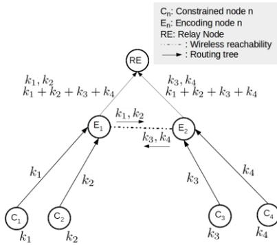
Fig. 2 Example of network coding at constrained network.
