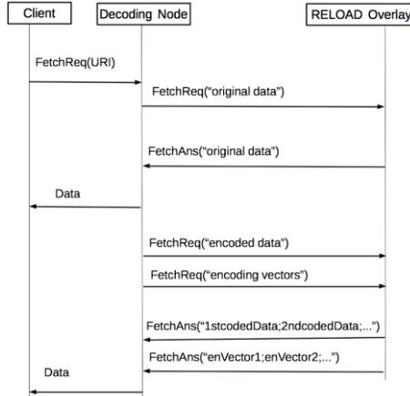
Fig. 3 Decoding at RELOAD/CoAP P2P overlay network.
