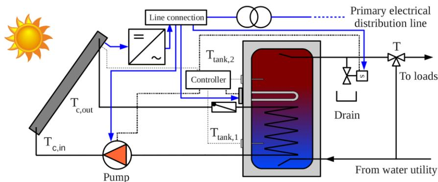
Fig. 1. Generic diagram for the solar domestic hot water (SDHW) systems studied.
