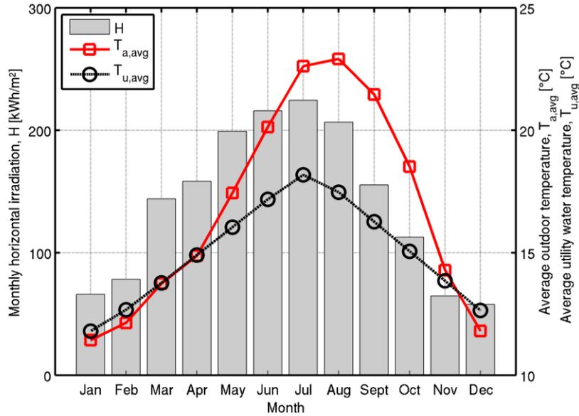
**Fig. 2.** Monthly horizontal irradiation ( $H$ ), average outdoor ( $T_{a,avg}$ ) and utility water temperatures ( $T_{u,avg}$ ) according to the (Lisbon) TMY data used in the simulations conducted.
