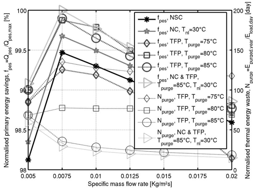
**Fig. 4.** Normalised primary energy savings ( $f_{pes}$ ) and normalised thermal energy waste due to fluid purging ( $N_{purge}$ ) versus the specific mass flow rate for the SDHW PV-T systems simulated. Legend: NSC, no stagnation control; NC, night cooling ( $T_{ni}=80^{\circ}\text{C}$ ; no load mode limited to vacations); TFP, tank fluid purging ( $T_{safe}=T_{purge}-5^{\circ}\text{C}$ ;  $m_{purge}=m_c$ ).
