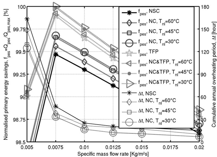
**Fig. 3.** Cumulative annual duration of overheating periods ( $\Delta t$ ) and normalised primary energy savings ( $f_{\text{pes}}$ ) versus the specific mass flow rate ( $m_c/A_c$ ) for the SDHW PV-T systems simulated. Legend: NSC, no stagnation control; NC, night cooling ( $T_n=80^\circ\text{C}$ ; no load mode limited to vacations, i.e., excludes weekends); TFP, tank fluid purging ( $T_{\text{purge}}=85^\circ\text{C}$ ;  $m_{\text{purge}}=m_c$ ).
