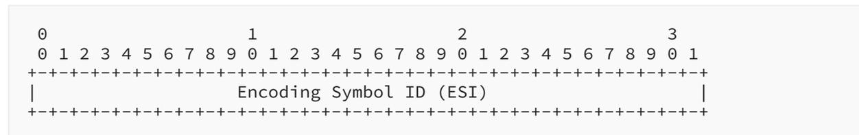
Figure 6: Source FEC Payload ID Encoding Format
