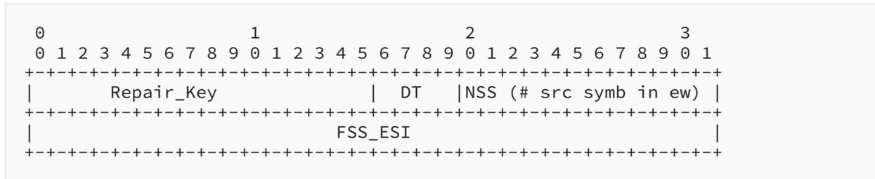
Figure 8: Repair FEC Payload ID Encoding Format
