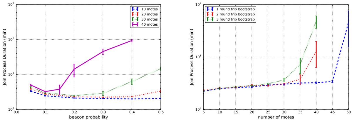
**FIGURE 2** a) Join duration for a single round trip bootstrap protocol and  $p_{DIO} = 1/3$ . For smaller values of  $p_{EB}$ , the dominant component of the duration is the time the mote spends unsynchronized waiting for EBs. For larger values (and increased traffic load) bootstrap retransmissions prevail. b) Join duration for beacon probability  $p_{EB} = 0.1$  and  $p_{DIO} = 1/3$ . For a given join process duration, the number of motes in the network decreases with increasing traffic load.
