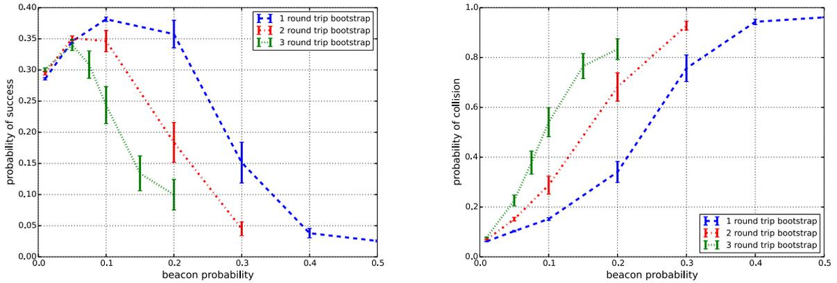
**FIGURE 1** a) Probability of success<sup>a)</sup> for a 40-mote fully-meshed network and  $p_{DIO} = 1/3$ .<sup>b)</sup> The increased bootstrapping load reduces the throughput during network formation process due to the increase in collisions. b) Probability of collision for a 40-mote fully-meshed network and  $p_{DIO} = 1/3$ . For optimal  $p_{EB} = 0.1$ , collisions double with increasing bootstrapping load.
