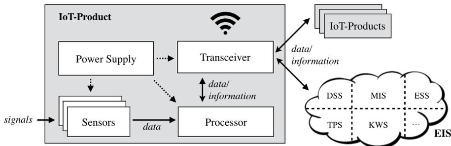
**Fig. 2.** Components of IoT-products necessary for product analytics
