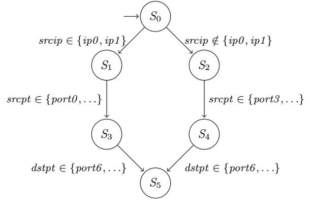
Figure 3. Data plane automaton for the toy example.
