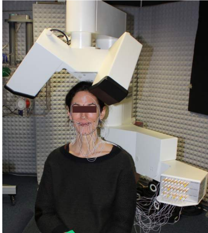
Figure 2: The articulo-graph AG501. A typical setting: The speaker is sitting under a block generating a low-intensity magnetic field. The sensors are glued on the face of the speaker. A unidirectional microphone is set in the front of the human speaker. The sensor movements and the speech signal are acquired synchronously.
