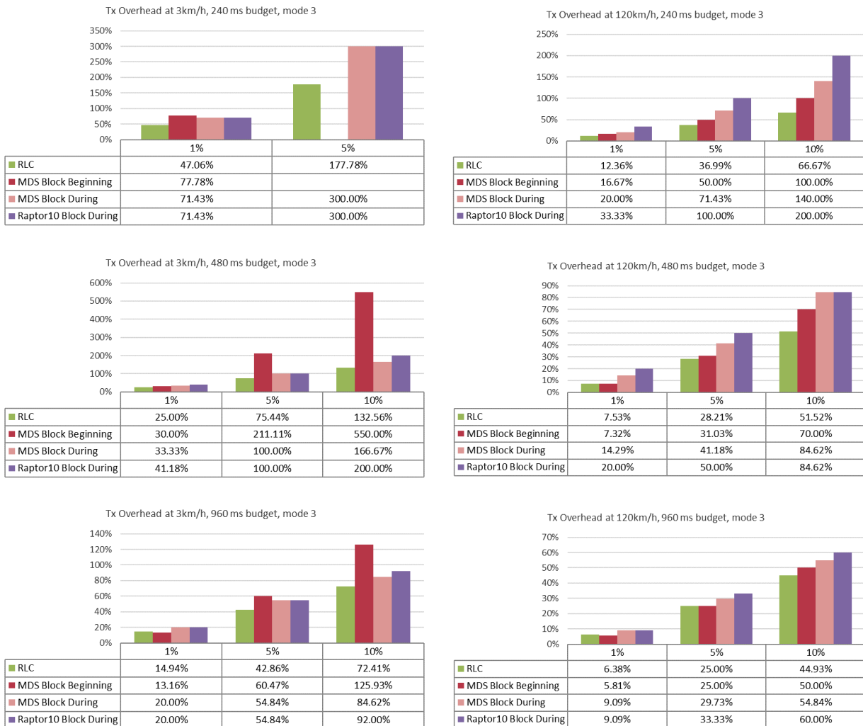
Figure 9.x.1.4.3-1 Repair traffic overhead for mode 3
