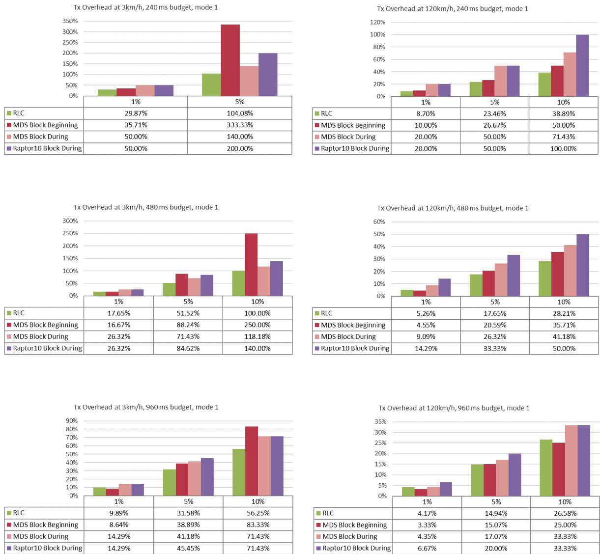
Figure 9.x.1.4.1-1 Repair traffic overhead for mode 1
