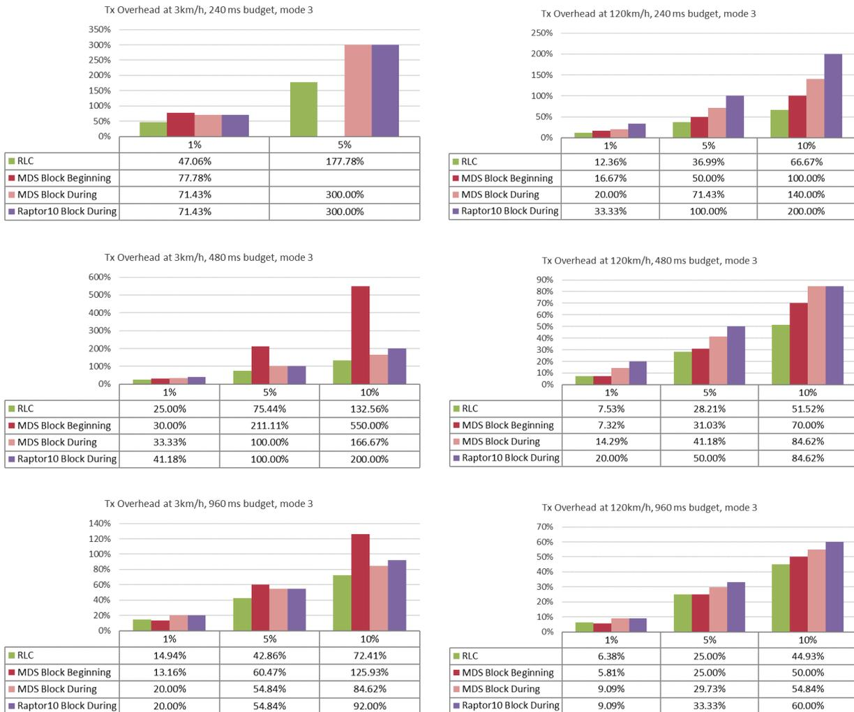
**Figure 9.x.1.4.3-1 Repair traffic overhead for mode 3**
