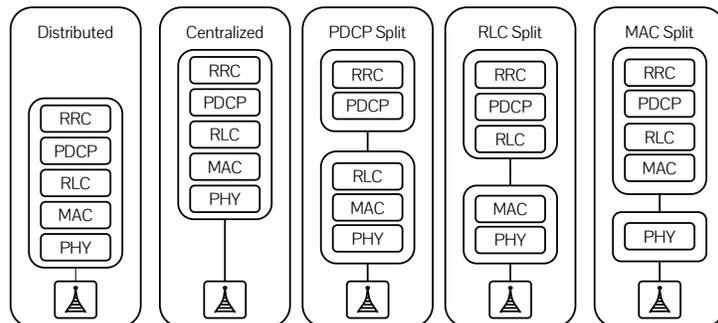
Fig. 1: Different functional splits for 5G small-cells [1].
