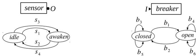
**Fig. 1.** Component models *sensor* (left) and *breaker* (right)
