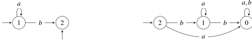
Figure 1: NFA \mathcal{A} recognizing the language L (left) and its reverse with added sink state 0 (right)
