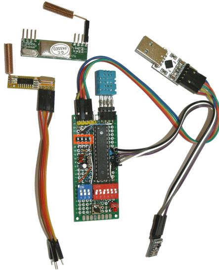
**Fig. 7.** Disassembled first prototype solution using ATMEGA 328P
