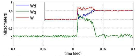
**Fig. 6:** response of the transducer to a step variation from  $1\mu m$  to  $1.5\mu m$
