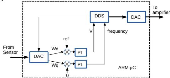
**Fig. 8:** The control scheme as embedded into a microcontroller
